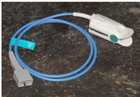
Hinged finger probe showing connector that can only be connected to the oximeter one way by aligning the gap on the probe connector with the corresponding notch on the machine.
