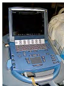
**Figure 4.** A micromax ultrasound machine
