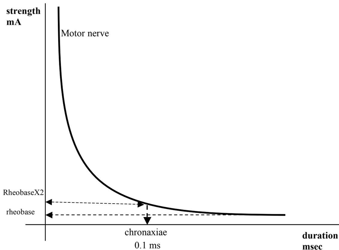
**Figure 2. Strength-duration curve for a motor nerve.** At a current equal to the rheobase the current has to be applied for a relatively long time. A current twice the rheobase value needs to be applied for a much shorter time to achieve a response.
