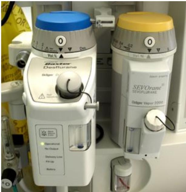
**Figure 6.** Desflurane (left) and sevoflurane (right) vapourisers.
